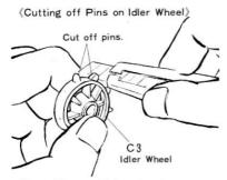
Fig. 4 Note in Fixing Wheels ★Though road wheels C5 and C4 are alike in shape, they are different in size of center holes. Also, C7 and C8 are different only in their hole diameter. Make sure of their number and fix.
